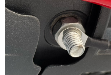
4 CONTROL GROUND + MAIN GROUND -> GROUND NEGATIVE
