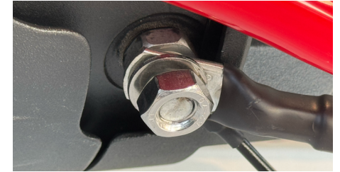
4 CONTROL GROUND + MAIN GROUND -> GROUND NEGATIVE
