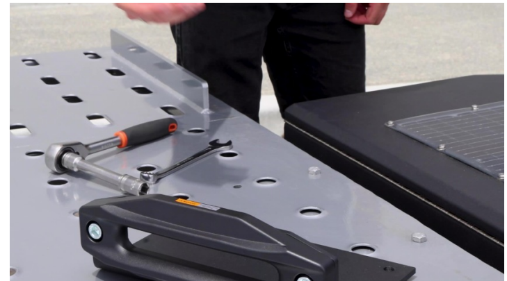
4 Tools required: Ratchet wrench, sockets (10mm, 16mm, 19mm), wrench, Phillips screwdriver
