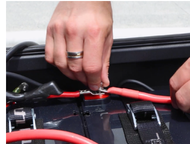
6 MAIN POSITIVE -> POSITIVE TERMINAL ON BATTERY (RECONNECT NEGATIVE AFTERWARD)
