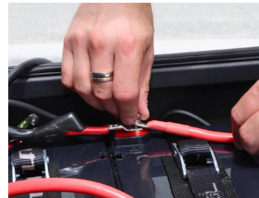
6 MAIN POSITIVE -> POSITIVE TERMINAL ON BATTERY (RECONNECT NEGATIVE AFTERWARD)
