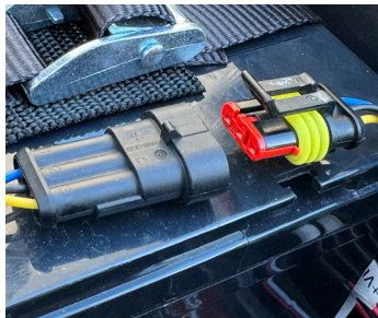
7 3-CORE CONTROL CABLE -> 3-CORE CONTROL CABLE PLUG (LABELLED RW)
