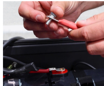
6 MAIN POSITIVE -> POSITIVE TERMINAL ON BATTERY (RECONNECT NEGATIVE AFTERWARD)
