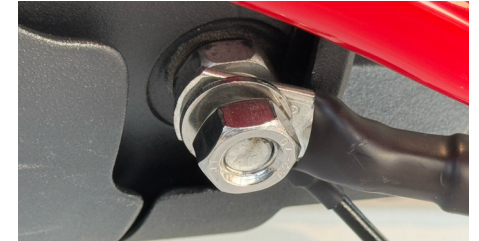
4 CONTROL GROUND + MAIN GROUND -> GROUND NEGATIVE
