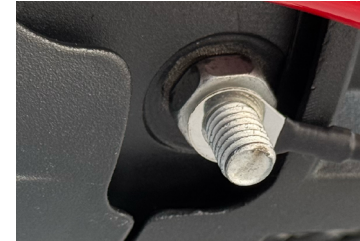
4 CONTROL GROUND + MAIN GROUND -> GROUND NEGATIVE
