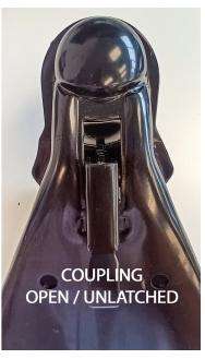
With the coupling open and in position over the tow hitch, release the handle and it will lock into place.
