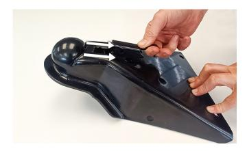
Position the coupling over the tow hitch and raise the handle up. With the handle raised and the coupling in position over the tow hitch, **slide the handle toward you** / away from the tow hitch to open the coupling.
