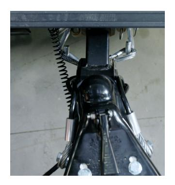
Connect to the tow vehicle. Ensure the safety cables and the break-away cable are securely connected to the tow vehicle.
