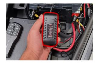
A 110V power adapter is supplied with the trailer to charge the battery when the trailer is stored.
