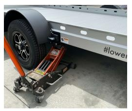
In case of trailer winch failure: If for any reason the winch fails to operate the trailer can be raised by placing a suitable jack under the mount beam and jacking from each side.
