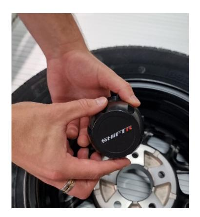
When fitting the SHITR Centre Cap on your Futura Trailer wheels, always check that it is positioned correctly.
