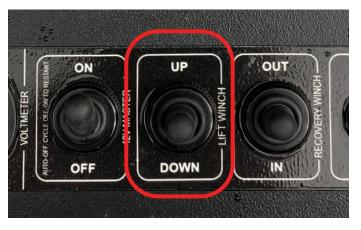
or - use the **SmartControl** manual switch to lower the trailer.
