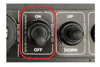
When the trailer is not in use, ensure the **SmartControl** master switch is turned off.
