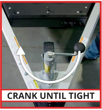
Crank up the jack wheel completely until the wheel locks.
