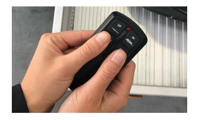
Turn on your **SmartControl** wireless remote by holding down the DOWN and OUT buttons simultaneously for 5 seconds until the red light illuminates.
