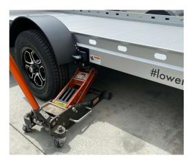
In case of trailer winch failure: If for any reason the winch fails to operate the trailer can be raised by placing a suitable jack under the mount beam and jacking from each side.
