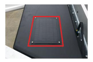
The trailer is equipped with a battery trickle charger which is powered by the tow vehicle auxiliary supply, if present on tow vehicle. The solar charger will operate in daylight to maintain the battery voltage.
