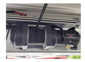
Regularly inspect the rope rigging. Ensure the winch rope is always neatly spooled on the winch drum. If any ropes are frayed, replace them immediately. Spare parts can be ordered online at <u>futuratrailers.com/my-futura</u>
