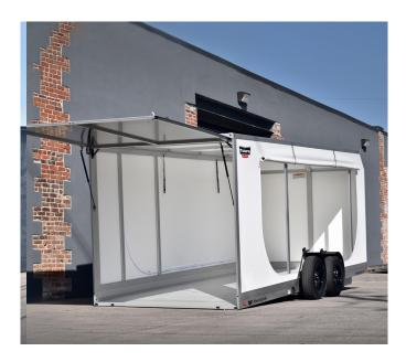
The sides should only be zipped open or closed when the trailer is fully raised and on level ground.
