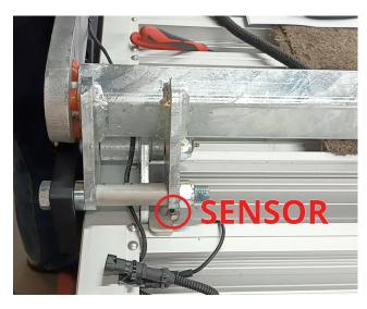
Step 3. Remove the allen cap screw from the left rear landing plate using the number 8 allen key and 17mm wrench.
