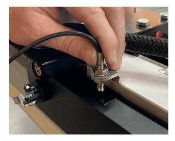
Step 7. Plug the sensor extension wiring into the sensor, ensuring the wiring runs between the chassis and the lifting rope (highlighted by red lines in the picture below). Plug the other end of the wiring into the sensor port.
