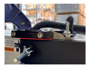
Step 11. Position the sensor set low in the bracket and using the 13mm wrenches, raise it up by adjusting the lock nuts until the light just goes off. When the sensor light goes off, the power to the trailer-raising-winch is cut off and the trailer stops raising. The sensor must be set so that the light goes off at the moment the lifting arms lands on the landing plate.
