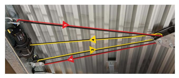
Step 1. From underneath the trailer, start by bolting the eyelet end of the Winch Rope to the shackle located to the right of the Trailer Raising Winch. IMPORTANT - secure shackle pin with medium strength thread locker - Loctite or similar.
