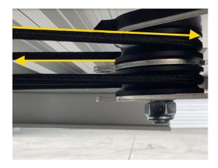
Step 5. Guide the rope back to the Trailer Raising Winch. Push the rope into the hole on the winch drum, so that it is flush with the drum, before securely tightening the set screw.
