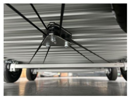
**ENSURE: LIFTING ARM ROPES ARE ABOVE AXLE - NO ROPES ARE CROSSED OR TWISTED**
