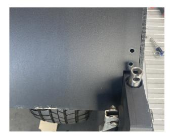
**Step 10.** Install the new fender latch mount over the fender latch hardware. Install one rivet in the bottom hole of the latch mount. Using a 5mm drill bit, drill through the top hole of the latch mount and through the fender before installing the second rivet.
