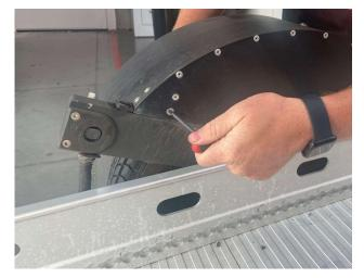
**Step 2.** Unplug the fender light plug and remove the fender.
