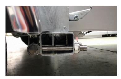
Apply low-strength Loctite to upper and lower nuts on the sensor. Proximity Sensor **MUST NOT** touch the Lifting Arm, there should be an air gap when the Lifting Arm has landed tight on the mount beam. The sensor is magnetic and the surface is easily damaged.
