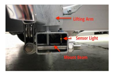
With the Lifting Arm resting flat on the Mount Beam, adjust the sensor height until indicator light on the sensor goes off. Replace the wheels and remove the supports so the load is on the wheels with the trailer on flat ground. Operate the winch and confirm the sensor stops the winch (indicator light goes off) just as the winch loads up and the Lifting Arm sits **TIGHT** on the Mount Beam.
