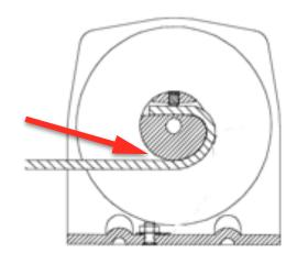
Hold tension on the rope and wind on **(UP)** so the rope lays neat on the winch drum.
