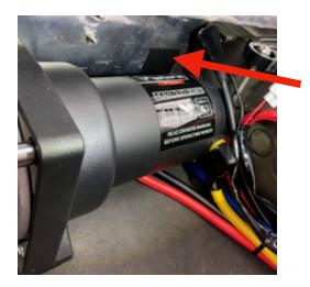
Place the plastic insulation card in the winch box above the winch electrical terminal. Slide the card down between the terminal and the back of the winch box.
