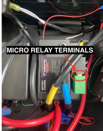
To short the Micro Relay terminals use the metal blade of a small screwdriver (or similar) with the Micro Relay connected to its base, prize the Micro Relay out just enough to get the small screw driver blade across the 2 terminals, 30 and 87, the Micro Relay must retain connection to the Micro Relay base.
