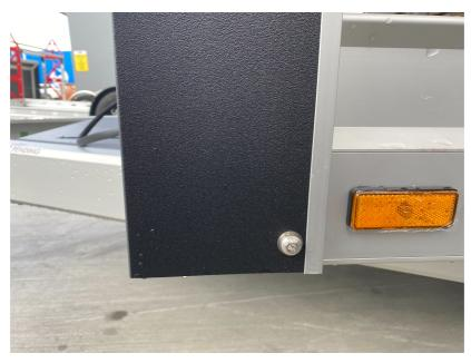
**Step 5:** Install the remaining 3 M10 X 50mm button screws into the 3 holes at the front of the trailer chassis.
