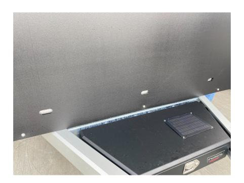
**Step 6:** Check that the Rock Guard has been properly mounted and sitting correctly. Check that all screws have been properly tightened.
