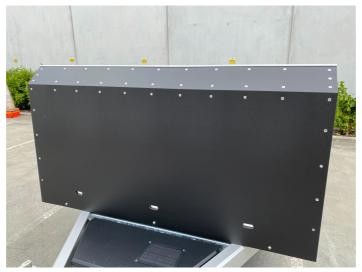
**Step 4:** Install the 2 side screws first (one on each side of the chassis) making sure they line up with the holes and rivnuts in the chassis. NOTE: You must ensure the holes line up as cross threading the screw in the rivnut mounted on the chassis can cause the rivnut to loosen from the chassis.
