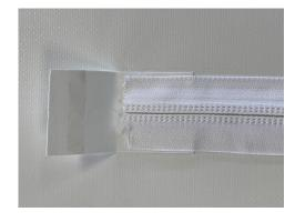
**Step 3.** Slide damaged slider out of zipper tape and replace with new slider.
